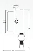
If left outlet required, invert Genie and use port labeled "BYPASS" as inlet, because sample must enter upper port.
