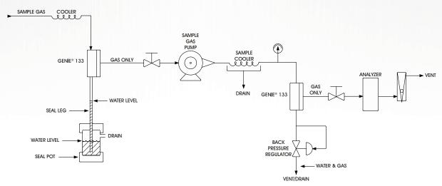
In the typical CEMS configuration shown above, Genie 133® separators provide protection to the sample gas pump against liquids upstream of the pump and protection to the analyzer against liquids and sulfuric acid aerosol upstream of the analyzer.
