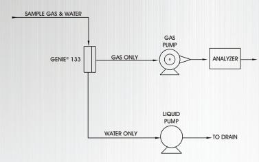
Sample gas and water enter the Genie® Membrane Separator™ via its inlet port where they are separated by the membrane. The gas (including water vapor) flows through the membrane, exits from the outlet port then on to the pump. Liquid water separated by the membrane gravity drains from the inlet cavity into tubing connected to a peristaltic pump. A timer can be used to periodically operate the pump.
