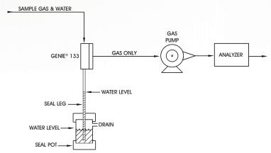
The Genie® Membrane Separator™ should be located at an elevation of three feet or greater that will allow for sufficient seal leg height. The height of the water column in the seal leg will be dependent upon the pump suction pressure, which, in typical sample systems, ranges from approximately 10 to 24 inches of water column below atmospheric pressure.
