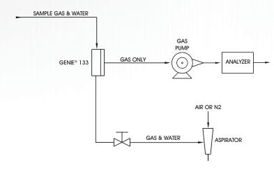
Sample gas and water enter the Genie® Membrane Separator™ via its inlet port where they are separated by the membrane. The gas (containing water vapor) flows through the membrane, exits from the outlet port then on to the pump.
