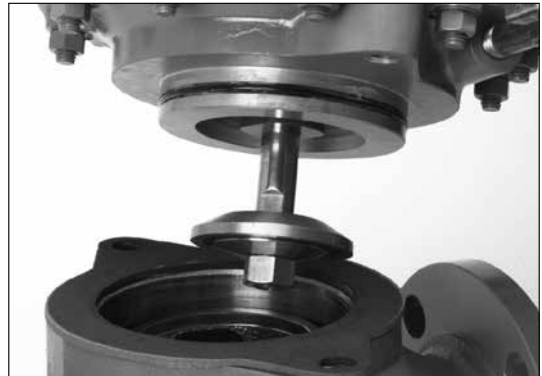
Figure 50 - Remove the actuator housing assembly
