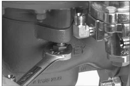
Figure 27 - Tightening the body cap screws
