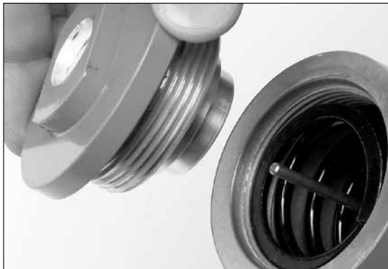
Figure 48 - Installing the spring case cap
