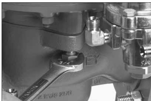
Figure 43 - Tightening the body cap screws
