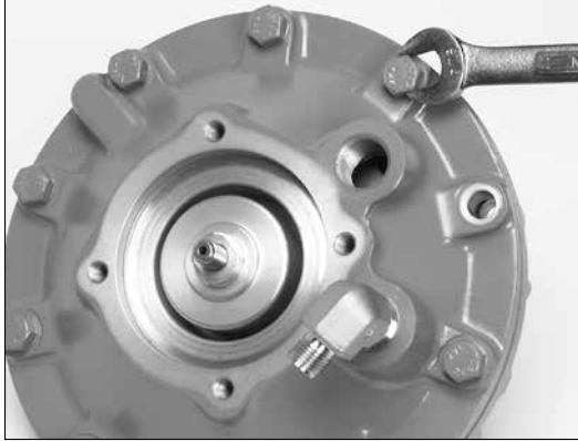
Figure 29 - Removing the housing cap screws
