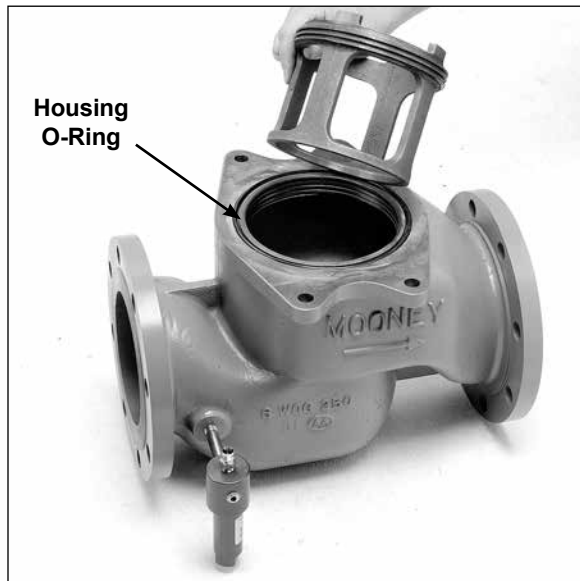
Figure 7b - 6" FlowMax: remove cage & inspect housing o-ring
