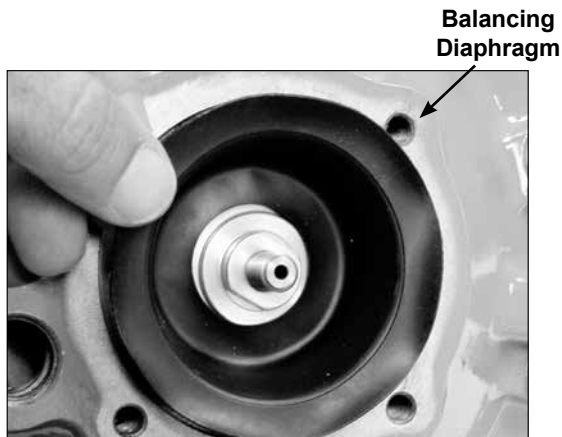
Figure 20 - Replacing the balancing diaphragm
