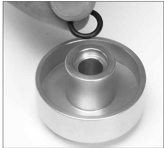
Figure 31 - Fig. 31 Inspecting stem o-ring
