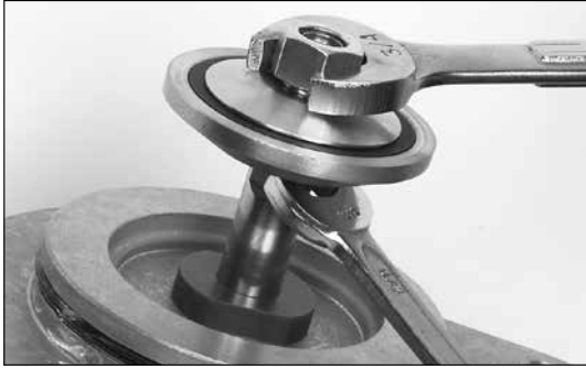
Figure 51 - Remove the stem nut
