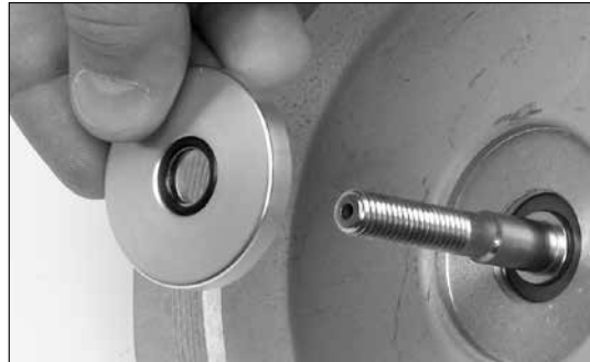
Figure 32 - Installing lower diaphragm retainer
