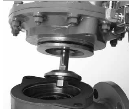
Figure 6 - Remove actuator from regulator body
