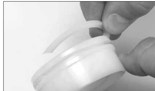
Figure 37 - Installing piston ring on piston
