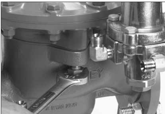
Figure 17 - Tightening the body cap screws
