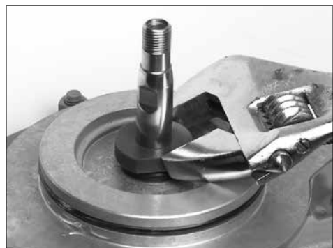
Figure 10 - Removing the stem bushing
