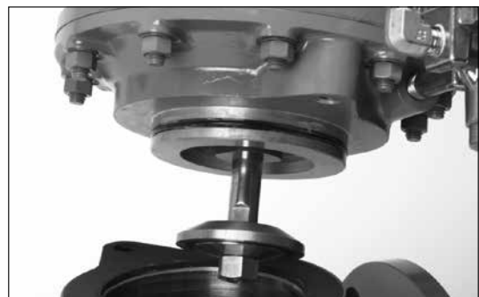
Figure 28 - Removing the main actuator
