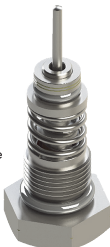
Figure 17 - Stack the Return Spring, Stem Guide, Orifice Spring, Plug and Stem, Orifice O-Ring, and Back up Washer on the Bottom Cap.
