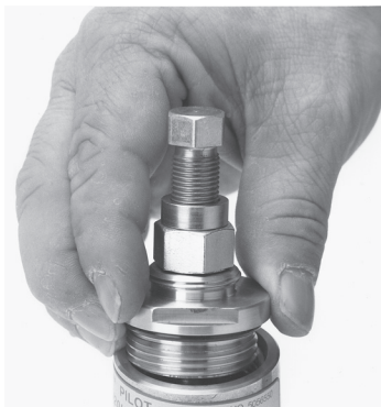
Figure 15 - Installing the closing cap assembly with spacer (to prevent spring over compression) for Pilots with the Black and White/Green Springs.
