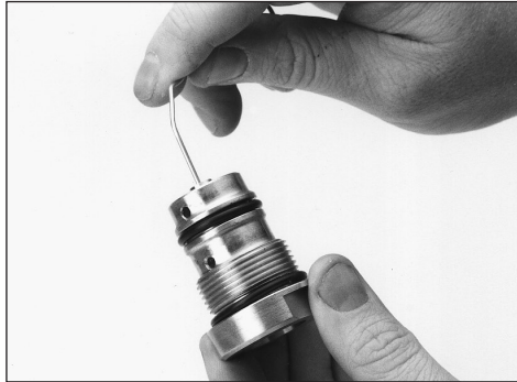
Figure 19 The orifice can be pushed out of the Body Insert (Cartridge) using a paper clip
