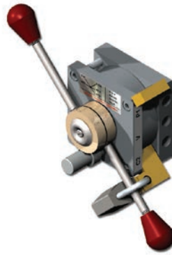
Figure 3.3 – MCV Optional Positioning Handle Locking Provision All MCV models are available with an optional positioning handle locking provision. This locking option allows the user to lock the control valve in either the full-open or full-closed position. This feature is useful during maintenance to provide lock out capabilities when it is desired to leave a valve in the full-open or full-closed position.
