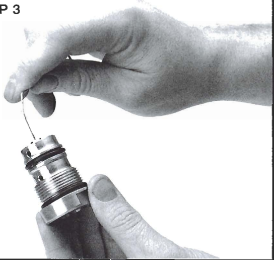
Figure 18. The orifice can be pushed out of the Body Insert (Cartridge) using a paper clip..
