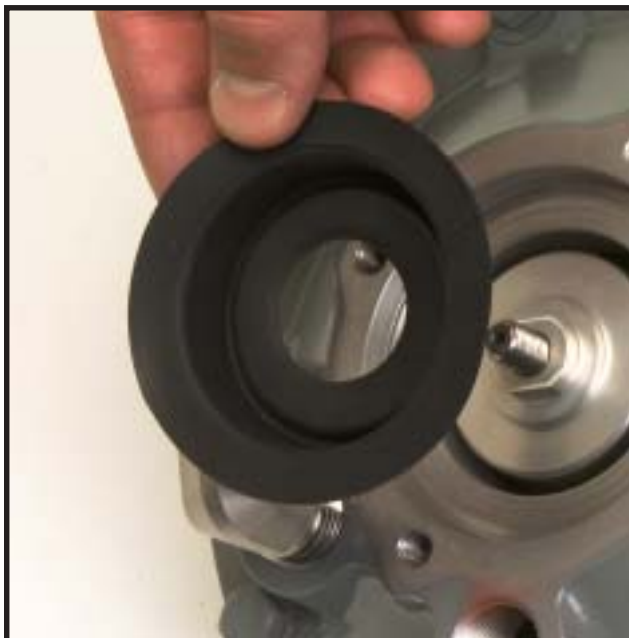
Fig. 35 Installing Balancing Diaphragm
