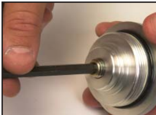
Fig. 45 Installing the Oring Retainer
