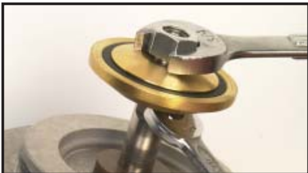
Fig. 13 Hold the Stem while tightening the Stem Nut
