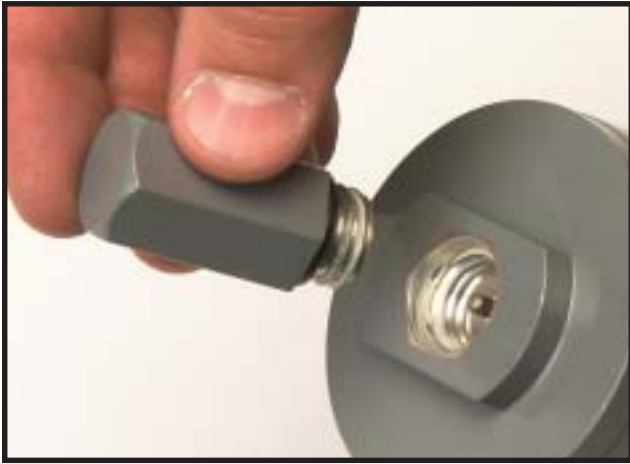
Fig. 47 Installing the Indicator Cover
