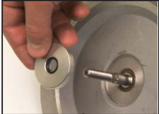
Fig. 32 Installing Lower Diaphragm Retainer
