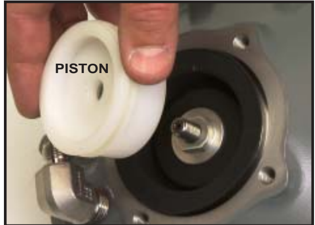
Fig. 36 Installing Piston on the Actuator Stem
