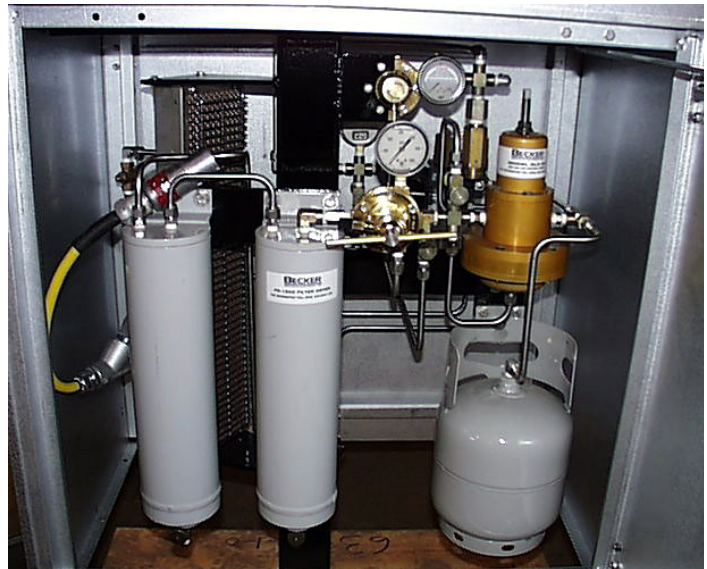
Figure x.0 - SLV-30 Signal Lock Valve post mounted inside of an enclosure complete with I/P Transducer, filtration, regulation, and heat provided by a catalytic heater. The complete assembly is for remote installation next to the actuator. An HPP Series Positioner is mounted directly on the actuator. The SLV senses the signal from the I/P and will keep the actuator in last position upon loss of that signal.
